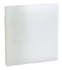
Stego filter, replacement, 6.61 x 6.61in, synthetic fiber, washable, G3 (coarse). Package of 5. For use with 6.93 x 6.93in Stego Filter Fan fans and exhaust grilles, Filter Fan Plus fans, and Filter Fan Plus FPO intake grilles.
