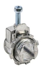
Halex fitting, zinc die cast, straight, 3/8in trade size, saddle conduit connection. Package of 50. For use with flexible metal conduit (FMC), AC cable (BX), MC cable, (NM-B) cable. Screws and locknut included.
