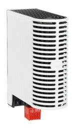
Stego enclosure heater, 150W heating capacity, touch-safe PTC resistor heating element, 120-240 VAC/VDC operating voltage, 50/60 Hz, fixed thermostat, N.C. (open on rise) 59 deg F (15 deg C) switch-on, 35mm DIN rail or panel mount.
