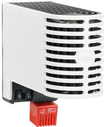
Stego enclosure heater, 50W heating capacity, touch-safe PTC resistor heating element, 120-240 VAC/VDC operating voltage, 50/60 Hz, fixed thermostat, N.C. (open on rise) 59 deg F (15 deg C) switch-on, 35mm DIN rail or panel mount.
