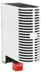
Stego enclosure heater, 150W heating capacity, touch-safe PTC resistor heating element, 120-240 VAC/VDC operating voltage, 50/60 Hz, fixed thermostat, N.C. (open on rise) 41 deg F (5 deg C) switch-on, 35mm DIN rail or panel mount.
