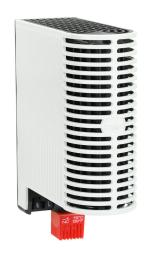
Stego enclosure heater, 100W heating capacity, touch-safe PTC resistor heating element, 120-240 VAC/VDC operating voltage, 50/60 Hz, fixed thermostat, N.C. (open on rise) 41 deg F (5 deg C) switch-on, 35mm DIN rail or panel mount.
