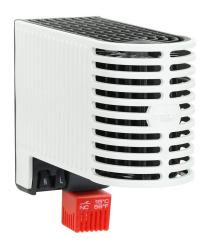
Stego enclosure heater, 50W heating capacity, touch-safe PTC resistor heating element, 120-240 VAC/VDC operating voltage, 50/60 Hz, fixed thermostat, N.C. (open on rise) 41 deg F (5 deg C) switch-on, 35mm DIN rail or panel mount.
