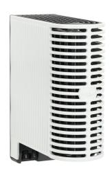
Stego enclosure heater, 150W heating capacity, touch-safe PTC resistor heating element, 120-240 VAC/VDC operating voltage, 50/60 Hz, 35mm DIN rail or panel mount.
