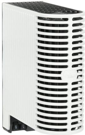
Stego enclosure heater, 100W heating capacity, touch-safe PTC resistor heating element, 120-240 VAC/VDC operating voltage, 50/60 Hz, 35mm DIN rail or panel mount.
