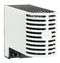
Stego enclosure heater, 50W heating capacity, touch-safe PTC resistor heating element, 120-240 VAC/VDC operating voltage, 50/60 Hz, 35mm DIN rail or panel mount.
