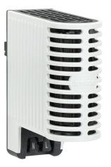
Stego enclosure heater, 30W heating capacity, touch-safe PTC resistor heating element, 120-240 VAC/VDC operating voltage, 50/60 Hz, 35mm DIN rail or panel mount.
