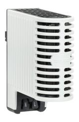
Stego enclosure heater, 30W heating capacity, touch-safe PTC resistor heating element, 120-240 VAC/VDC operating voltage, 50/60 Hz, 35mm DIN rail or panel mount.
