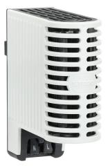
Stego enclosure heater, 20W heating capacity, touch-safe PTC resistor heating element, 120-240 VAC/VDC operating voltage, 50/60 Hz, 35mm DIN rail or panel mount.
