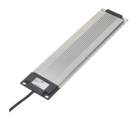
Stego flat heater, 100W heating capacity, PTC resistor heating element, 230 VAC operating voltage, 50/60 Hz, M6 screw mount.
