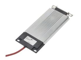
Stego flat heater, 50W heating capacity, resistance heating element, 120 VAC operating voltage, 50/60 Hz, M6 screw mount.
