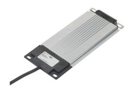
Stego flat heater, 50W heating capacity, resistance heating element, 230 VAC operating voltage, 50/60 Hz, M6 screw mount.
