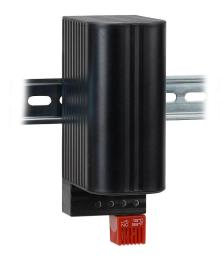
Stego enclosure heater, 150W heating capacity, touch-safe PTC resistor heating element, 120-240 VAC operating voltage, fixed thermostat, N.C. (open on rise) 41 deg F (5 deg C) switch-on, 35mm DIN rail mount.
