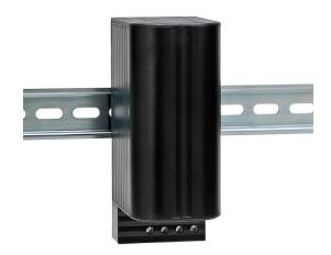
Stego enclosure heater, 150W heating capacity, touch-safe PTC resistor heating element, 120-240 VAC/VDC operating voltage, 35mm DIN rail mount.
