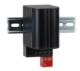
Stego heater, 100W heating capacity, touch-safe PTC resistor heating element, 120-240 VAC operating voltage, fixed thermostat, N.C. (open on rise) 41 deg F (5 deg C) switch-on, 35mm DIN rail mount.
