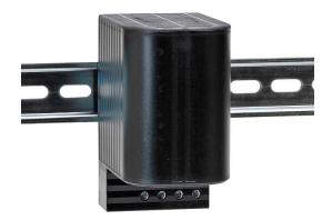
Stego enclosure heater, 100W heating capacity, touch-safe PTC resistor heating element, 120-240 VAC/VDC operating voltage, 35mm DIN rail mount.
