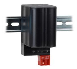
Stego enclosure heater, 50W heating capacity, touch-safe PTC resistor heating element, 120-240 VAC operating voltage, fixed thermostat, N.C. (open on rise) 41 deg F (5 deg C) switch-on, 35mm DIN rail mount.
