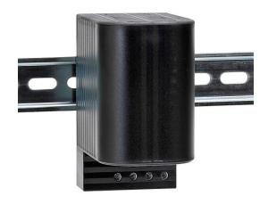
Stego enclosure heater, 50W heating capacity, touch-safe PTC resistor heating element, 120-240 VAC/VDC operating voltage, 35mm DIN rail mount.
