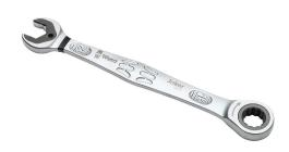
Wera Joker combination wrench, ratcheting, 12mm, 7.4in (188mm) overall length, special nut holding feature and fine tooth ratchet.
