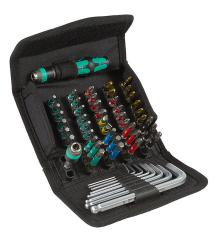
Wera Kraftform Kompakt standard and impact driver bit set, Phillips, Pozidriv, Torx, slotted and external hex, 52 pieces, 1in and 2in bit length, 1/4in drive, metric.
