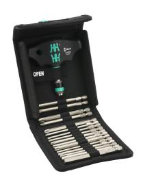
Wera Kraftform Kompakt standard T-handle bit holder set, Phillips, Pozidriv, Torx, external hex and slotted, 17 pieces, 3.5in bit length, 1/4in drive, metric.
