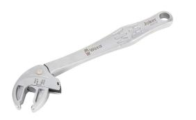
Wera Joker adjustable wrench, ratcheting, 1/2-5/8in, 7.5in (190mm) overall length, automatic and continuous self-setting, 30 degree low return angle and contactless jaw opening feature.
