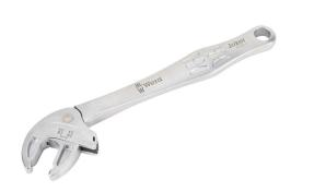
Wera Joker adjustable wrench, ratcheting, 5/8-3/4in, 8.9in (226mm) overall length, automatic and continuous self-setting, 30 degree low return angle and contactless jaw opening feature.
