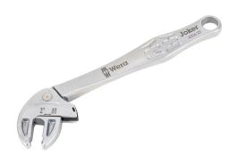
Wera Joker adjustable wrench, ratcheting, 1/4-3/8in, 4.7in (119mm) overall length, automatic and continuous self-setting, 30 degree low return angle and contactless jaw opening feature.
