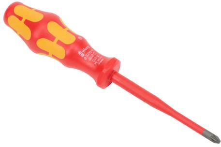
Wera Kraftform Plus #2 Pozidriv insulated screwdriver, 1000V insulation rating, 3.9in (100mm) shaft length, reduced shank, Kraftform ergonomic handle.
