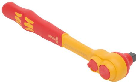
Wera Zyklop VDE ratchet, insulated, switch lever, 3/8in drive, 4.5 degrees return angle, Kraftform ergonomic handle, 90-degree fixed head, metal with plastic coating construction, ballpoint socket with button release mechanism locking mechanism.
