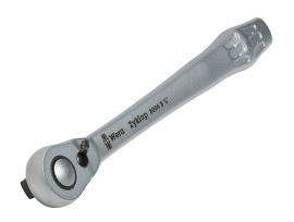
Wera Zyklop Metal ratchet, switch lever, 3/8in drive, 5 degrees return angle, all-metal construction, ballpoint socket locking mechanism.
