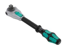
Wera Zyklop Speed ratchet, dial switch, 1/2in drive, 5 degrees return angle, Kraftform ergonomic handle, locking swivel head, free-turning sleeve, ballpoint socket locking mechanism.
