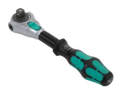
Wera Zyklop Speed ratchet, dial switch, 3/8in drive, 5 degrees return angle, Kraftform ergonomic handle, locking swivel head, free-turning sleeve, ballpoint socket locking mechanism.
