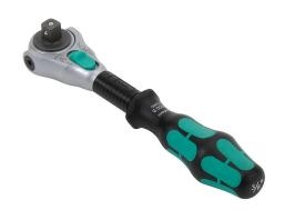
Wera Zyklop Speed ratchet, dial switch, 3/8in drive, 5 degree return angle, Kraftform ergonomic handle, locking swivel head, free-turning sleeve, secure socket lock mechanism. Manufacturer part number: 003550.
