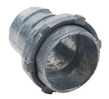
Halex fitting, zinc die cast, straight, 1-1/2in trade size, twist-in conduit connection. Package of 10. For use with flexible metal conduit (FMC). Locknut included.
