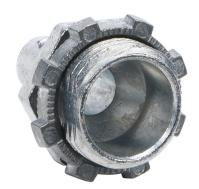
Halex fitting, zinc die cast, straight, 3/8in trade size, twist-in conduit connection. Package of 50. For use with flexible metal conduit (FMC). Locknut included.
