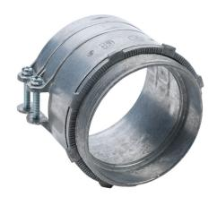
Halex fitting, zinc die cast, straight, 4in trade size, squeeze conduit connection. Package of 1. For use with flexible metal conduit (FMC). Screw and locknut included.
