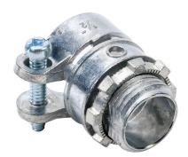
Halex fitting, zinc die cast, straight, 1/2in trade size, squeeze conduit connection. Package of 25. For use with flexible metal conduit (FMC), AC cable (BX), MC cable. Screw and locknut included.
