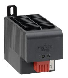
Stego enclosure heater, axial fan, 1000W heating capacity, PTC resistor heating element, 100-120 VAC operating voltage, 50/60 Hz, fixed thermostat, N.C. (open on rise) 41 deg F (5 deg C) switch-on, panel mount.
