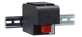
Stego enclosure heater, axial fan, 1000W heating capacity, PTC resistor heating element, 100-120 VAC operating voltage, 50/60 Hz, fixed thermostat, N.C. (open on rise) 41 deg F (5 deg C) switch-on, 35mm DIN rail mount.
