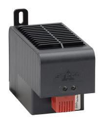
Stego enclosure heater, axial fan, 1000W heating capacity, PTC resistor heating element, 220-240 VAC operating voltage, 50/60 Hz, fixed thermostat, N.C. (open on rise) 41 deg F (5 deg C) switch-on, panel mount.
