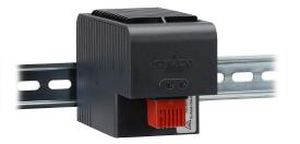
Stego enclosure heater, axial fan, 1000W heating capacity, PTC resistor heating element, 220-240 VAC operating voltage, 50/60 Hz, fixed thermostat, N.C. (open on rise) 41 deg F (5 deg C) switch-on, 35mm DIN rail mount.
