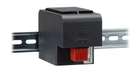
Stego enclosure heater, axial fan, 1000W heating capacity, PTC resistor heating element, 220-240 VAC operating voltage, 50/60 Hz, fixed thermostat, N.C. (open on rise) 41 deg F (5 deg C) switch-on, 35mm DIN rail mount.
