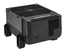
Stego enclosure heater, axial fan, 800W heating capacity, high performance cartridge heating element, 56 VDC operating voltage, adjustable thermostat, N.C. (open on rise) -4 to 104 deg F, foot mount.
