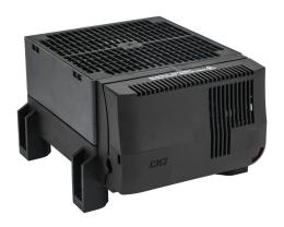
Stego enclosure heater, axial fan, 200W heating capacity, high performance cartridge heating element, 24 VDC operating voltage, adjustable thermostat with external sensor connection, N.C. (open on rise) -4 to 104 deg F, foot mount.
