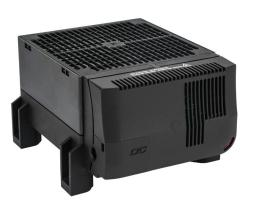
Stego enclosure heater, axial fan, 200W heating capacity, high performance cartridge heating element, 24 VDC operating voltage, adjustable thermostat, N.C. (open on rise) -4 to 104 deg F, foot mount.
