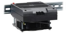
Stego enclosure heater, axial fan, 500W heating capacity, high performance cartridge heating element, 120 VAC operating voltage, 50/60 Hz, 35mm DIN rail mount.
