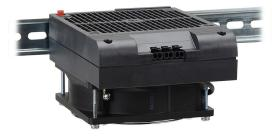
Stego enclosure heater, axial fan, 600W heating capacity, high performance cartridge heating element, 120 VAC operating voltage, 50/60 Hz, 35mm DIN rail mount.
