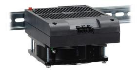
Stego enclosure heater, axial fan, 700W heating capacity, high performance cartridge heating element, 120 VAC operating voltage, 50/60 Hz, 35mm DIN rail mount.
