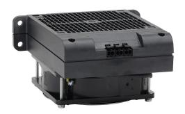
Stego enclosure heater, axial fan, 700W heating capacity, high performance cartridge heating element, 230 VAC operating voltage, 50/60 Hz, panel mount.
