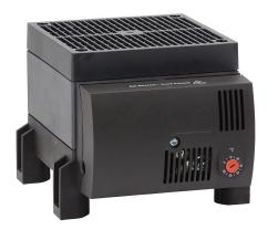
Stego enclosure heater, axial fan, 1200W heating capacity, PTC resistor heating element, 230 VAC operating voltage, 50/60 Hz, adjustable thermostat, N.C. (open on rise) 0 to 60 deg C, foot mount.
