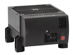
Stego enclosure heater, axial fan, 950W heating capacity, high performance cartridge heating element, 230 VAC operating voltage, 50/60 Hz, adjustable thermostat, N.C. (open on rise) 0 to 60 deg C, foot mount.
