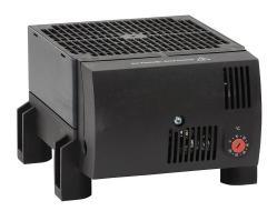
Stego enclosure heater, axial fan, 950W heating capacity, high performance cartridge heating element, 230 VAC operating voltage, 50/60 Hz, adjustable thermostat, N.C. (open on rise) 0 to 60 deg C, foot mount.
