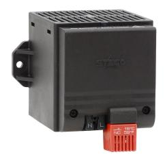
Stego enclosure heater, axial fan, 250W heating capacity, touch-safe PTC resistor heating element, 230 VAC operating voltage, 50/60 Hz, fixed thermostat, N.C. (open on rise) 41 deg F (5 deg C) switch-on, panel mount.
