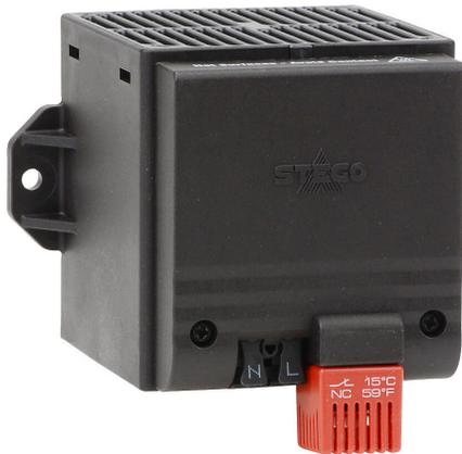
Stego enclosure heater, axial fan, 250W heating capacity, touch-safe PTC resistor heating element, 230 VAC operating voltage, 50/60 Hz, fixed thermostat, N.C. (open on rise) 41 deg F (5 deg C) switch-on, panel mount.
